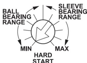
After you begin at the recommended setting, you can fine tune the hard start time within the recommended range for the type of motor you have.
