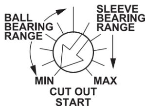
**CAUTION!:** With sleeve bearing motors, it is important not to adjust outside the sleeve bearing range or bearing failure may result.
