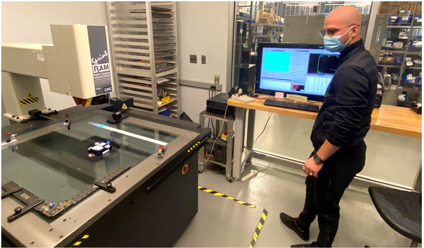
With the optical video probe (OVP), Operator Julio Placeres gathers detailed full-color images.
