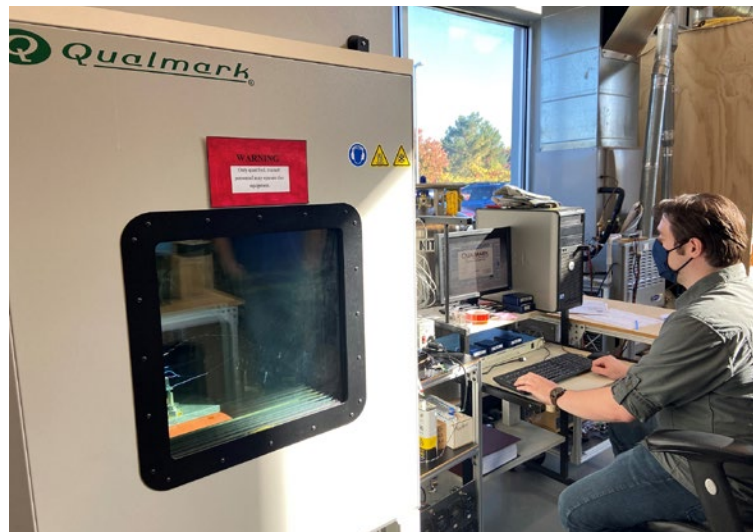
Operator Dan Kranze conducting a highly accelerated life test (HALT).
