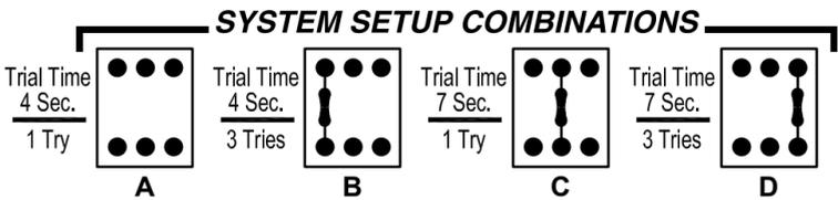
**IMPORTANT:** It is best to remove the jumpers before installing the ICM283. Do not cut the jumpers with power applied to the control. Completely remove unneeded jumpers. Carefully cut the jumper with wire cutters and discard the jumper.
