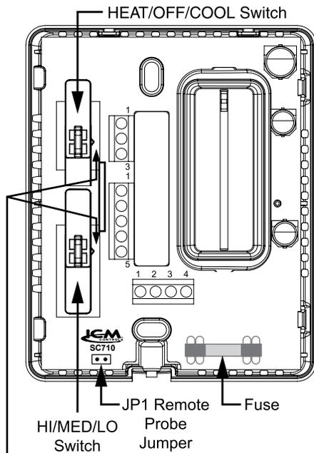
**NOTE:** Switch caps must be installed with point in this position to insure proper operation.
