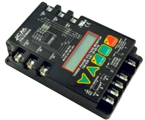
The ICM450 was specifically designed to protect motors and other 3-phase loads from premature failure and damage due to common voltage faults such as voltage unbalance, over/under voltage, phase loss, reversal, incorrect sequencing and rapid short cycling.
