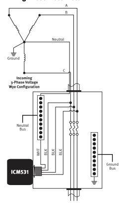
Type 2 Wiring - Circuit Breaker
