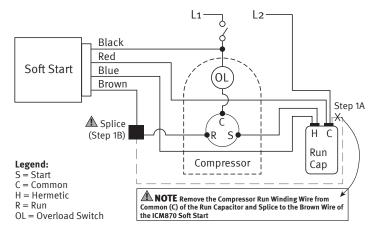
Special attention should be made with respect to the termination of the field wiring leads, only at terminals suitable for a 90°C wire at minimum.
